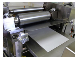
Paper coating with NFC/ZnO composites to obtain antibacterial papers
